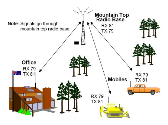
Figure 3: Repeater radio operations
