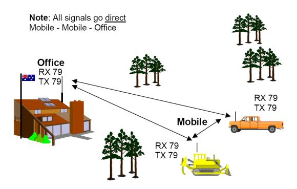
Figure 2: Simplex radio operations
